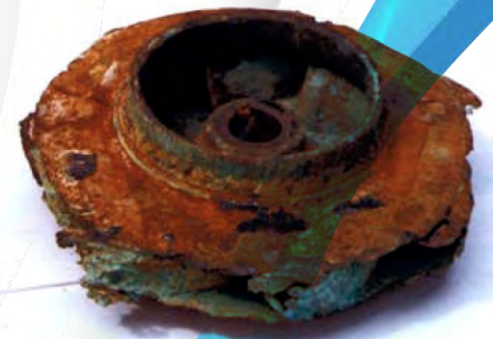
Discharge Recirculation Cavitation
