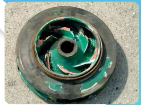
Suction Recirculation Cavitation: Damage in fresh water after only 3 months of operation!
