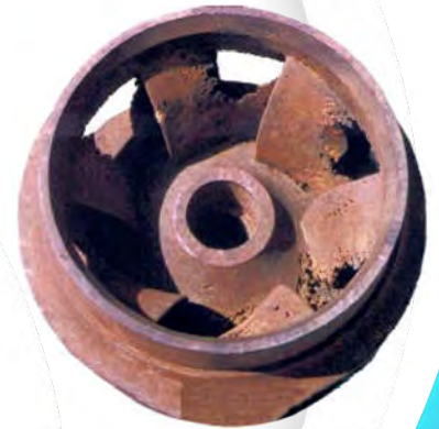
Suction Recirculation Cavitation damage.
